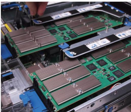
Photo 4. PCI Express Riser Card Re-installation
